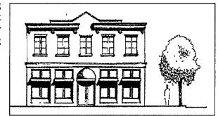
The minimum window and door requirements are measured between 2 and 8 feet from the ground. Only the glass portion of doors may be used in the calculation.
