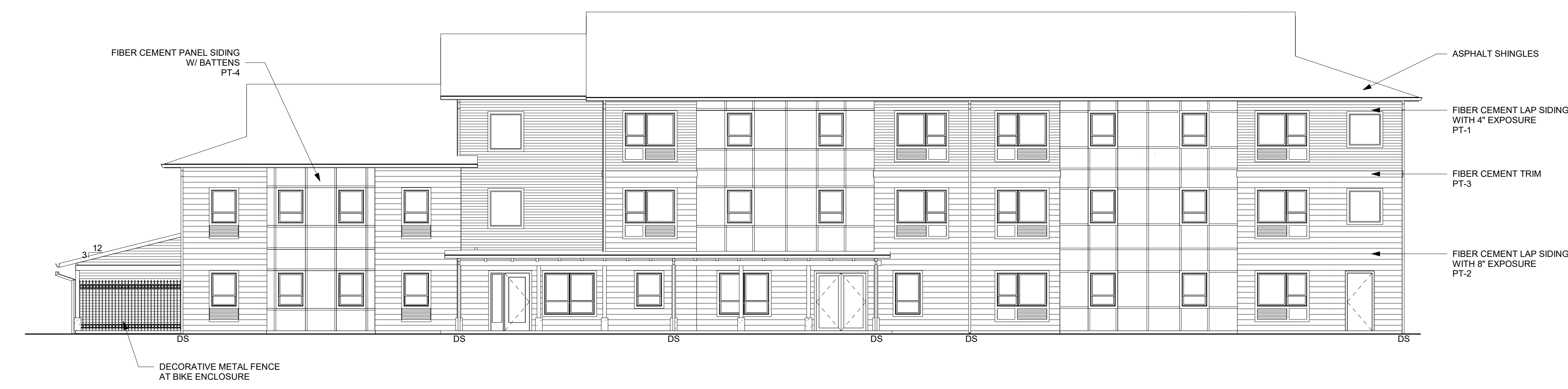
3 BUILDING ELEVATION - EAST 1/8" = 1'-0"
