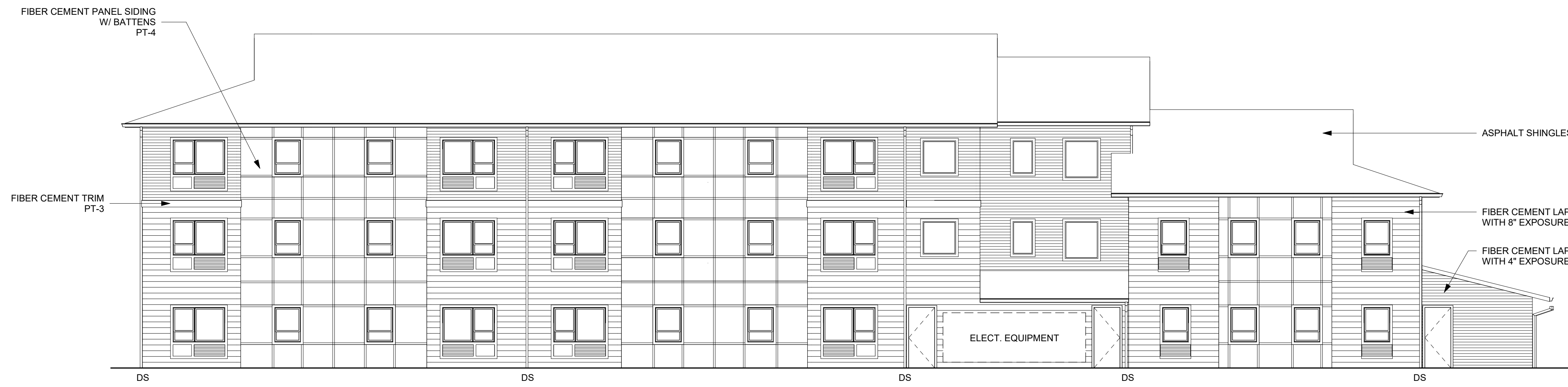
4 BUILDING ELEVATION - WEST 1/8" = 1'-0"
