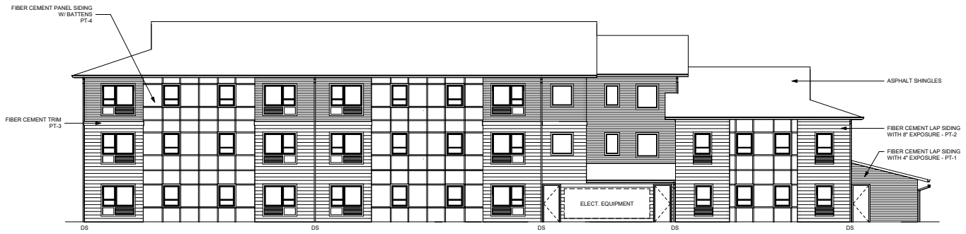
4 BUILDING ELEVATION - WEST A211 1/8" = 1'-0"
